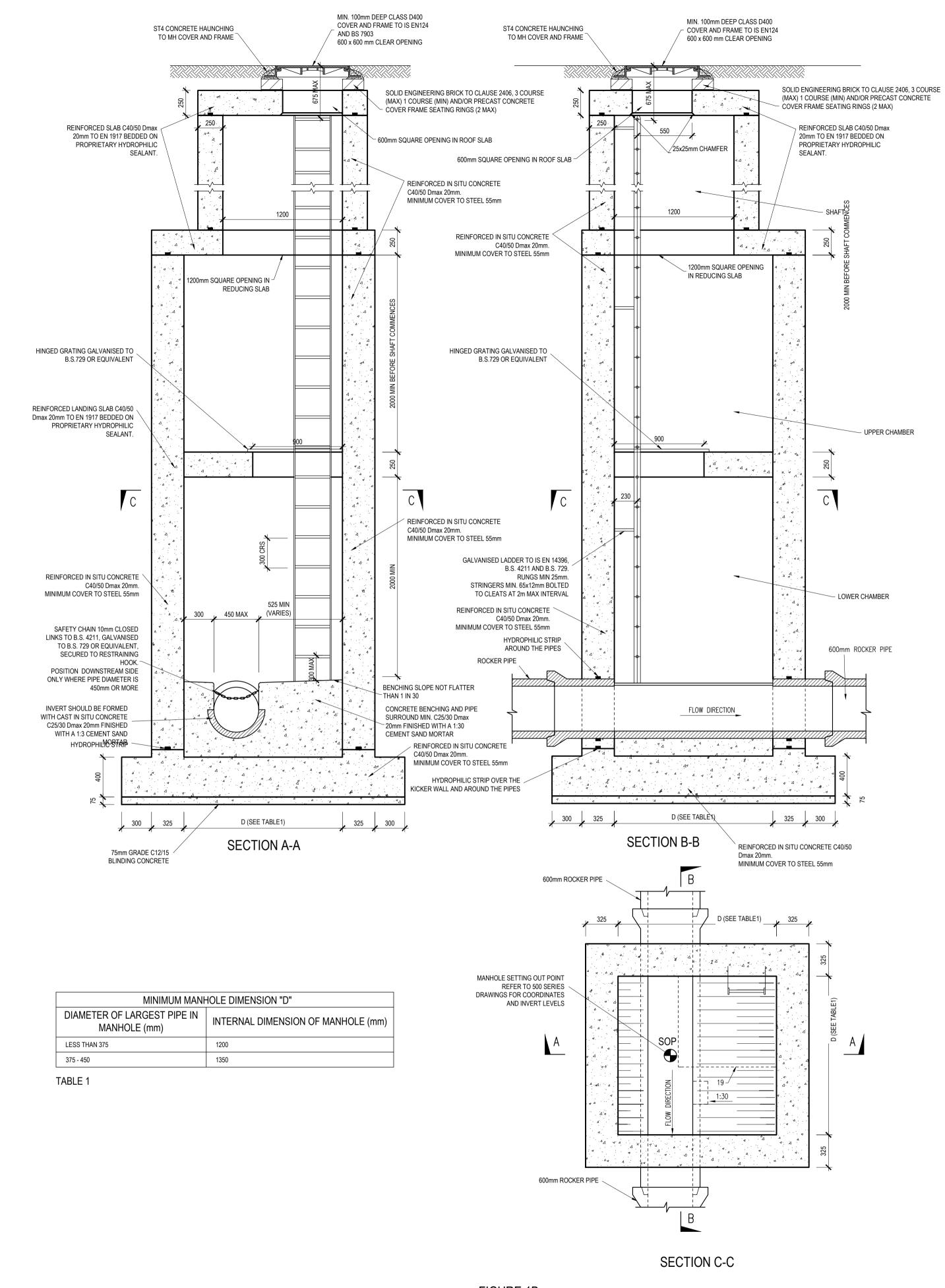
FIGURE 1B TYPICAL FW MANHOLE DETAIL FOR PIPE DIAMETERS 225,300,375 & 450 DEPTH TO INVERT 6 TO 8m SCALE 1:25
